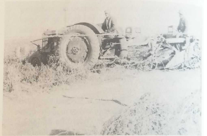
An early tractor drawing a corn binder. This tractor has rubber tires.
